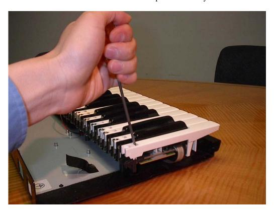
4.23 Use the screwdriver to bend the tab inside the key while pushing the key forward and up.
